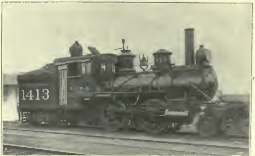
FIG. 383. LOCOMOTIVES. Suburban Passenger Locomotive of the Forney Type. Illinois Cen- tral Railroad.
